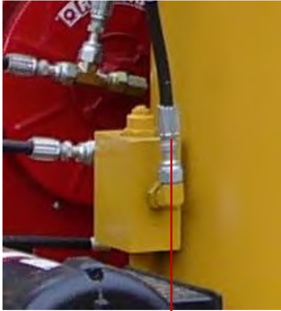
6. Remove this hose from here. This is the extend port which varies from machine to machine. On some systems this port is on the left hand side of the valve body. And the pilot and test port are on the right side.
