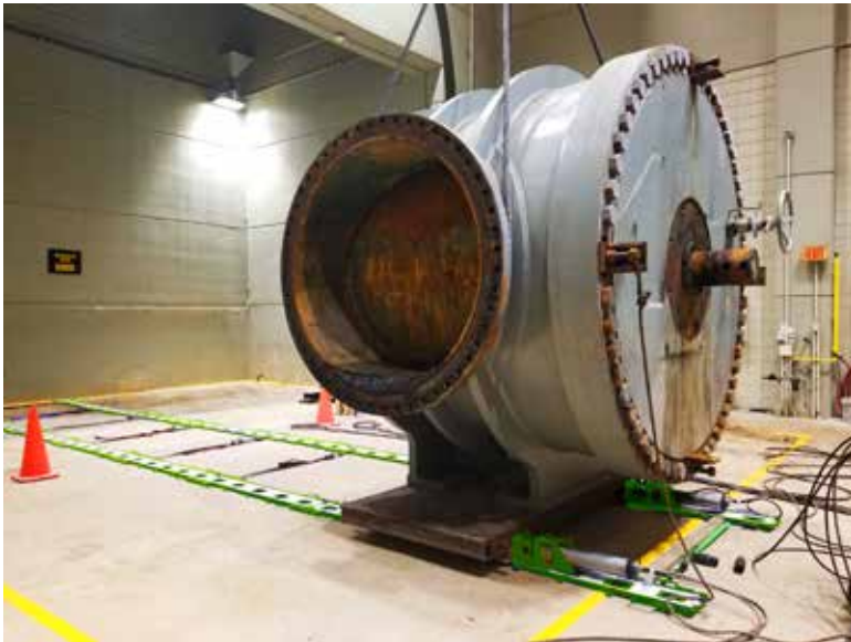
LP350 Example - the load is supported on two 3' sections, with full support under the track:
