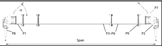
Typical Spreader Assembly
