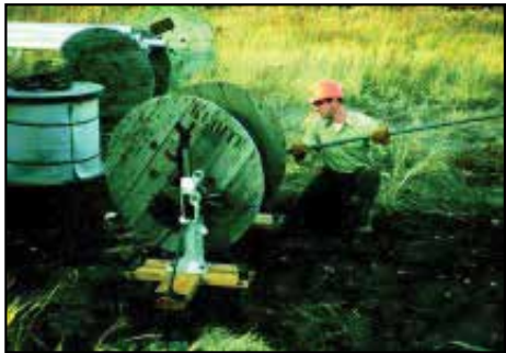
Using A1029-R and A1029-L, utilities can easily handle large reels. The large wooden bases and low handle efforts enhance safety and reduce operator fatigue. Simplex Reel Jacks are also an excellent choice for wire rope and sling manufacturers.
